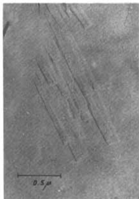
Figure 2a. Electron micrograph of single crystals of TMA grown at room temperature in a solvent-non-solvent mixture of dioxane and 60% octane
