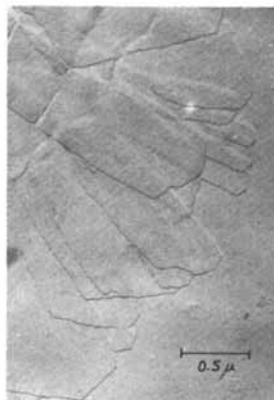
Figure 2b. Electron micrograph of single crystals of TMA grown at 180°–150°C in diethyleneglycol
